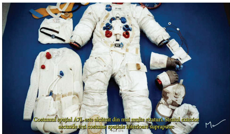
Fig. 8. Structural overview of the Apollo A7L suit and its components
